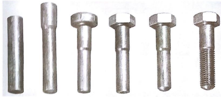
FIGURE 19-9 Steps in the forming of a bolt by cold extrusion, cold heading, and thread rolling. (Courtesy of National Machinery Co.)
